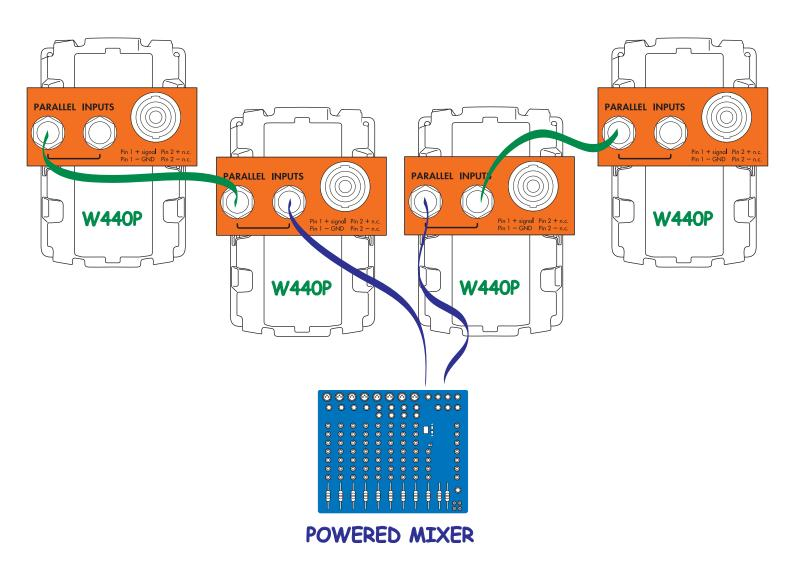
MIXER L/R POWERED OUTPUTS W440P INPUTS W440P OUTPUTS INPUTS of other W440P
